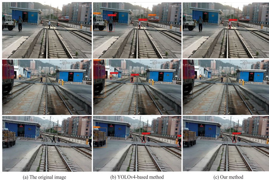
FIGURE 7. Comparison of the YOLOv4-based method and our detector.
