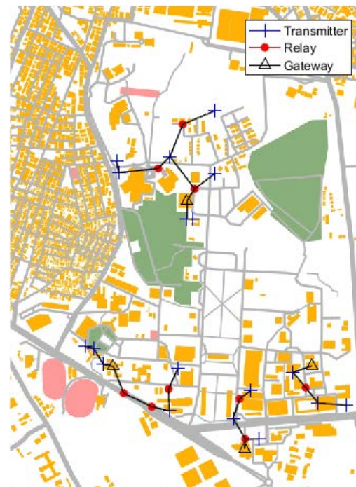
FIGURE 6. Network design for four gateways and multiple transmitters in a heterogeneous region.
