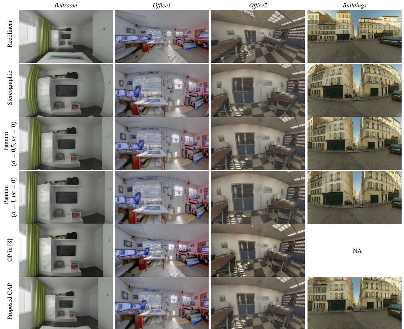
FIGURE 18. Example of viewports rendered from a different ERI with different projections using horizontal FoV of 150°. The proposed CAP produces viewports more pleasant than the other projections.
