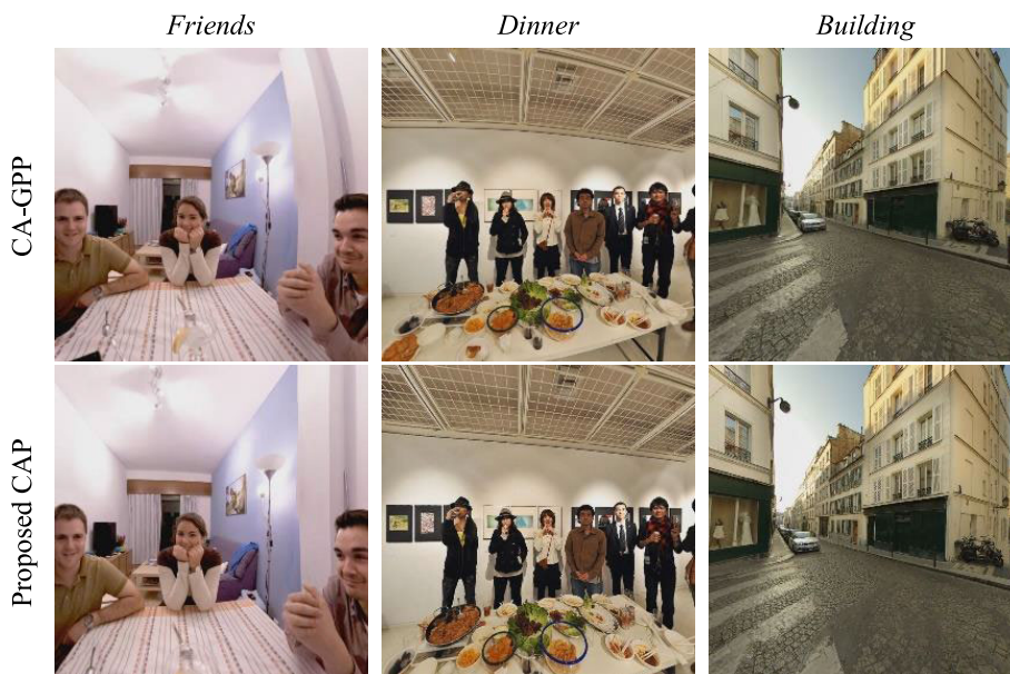
FIGURE 19. Example of viewports rendered from a different ERI with proposed CAP and CA-GPP using a square FoV of 110°. The proposed CAP produces viewports with less geometric deformations, lines are straighter and the object shapes are less deformed.
