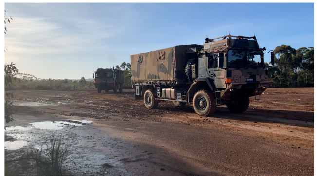
FIGURE 8. Driving on a dirt road: An autonomous convoy needs the capability of operating on not just quality tarred roads but also dirt roads without markings (Photograph taken during a project demonstration with the Australian Army).
