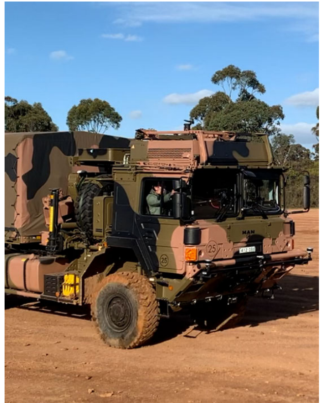
FIGURE 9. Proof of autonomy by lifting hands by a driver (who takes over vehicle control only during emergencies) while the military truck moves on a dirt road (Photograph taken during a project demonstration with the Australian Army).
