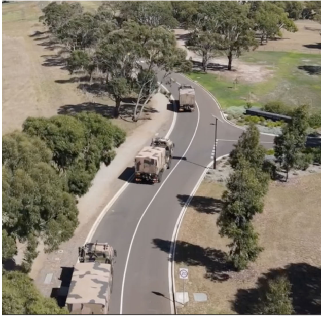
FIGURE 1. An example of autonomous convoying of military trucks consisting of a leader and two followers (Photograph taken during a project demonstration with the Australian Army).
