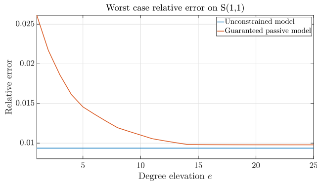
FIGURE 20. High-speed link. Evolution of the relative error \epsilon_{1,1} for the passive models with different degree elevations, compared to the unconstrained model error.
