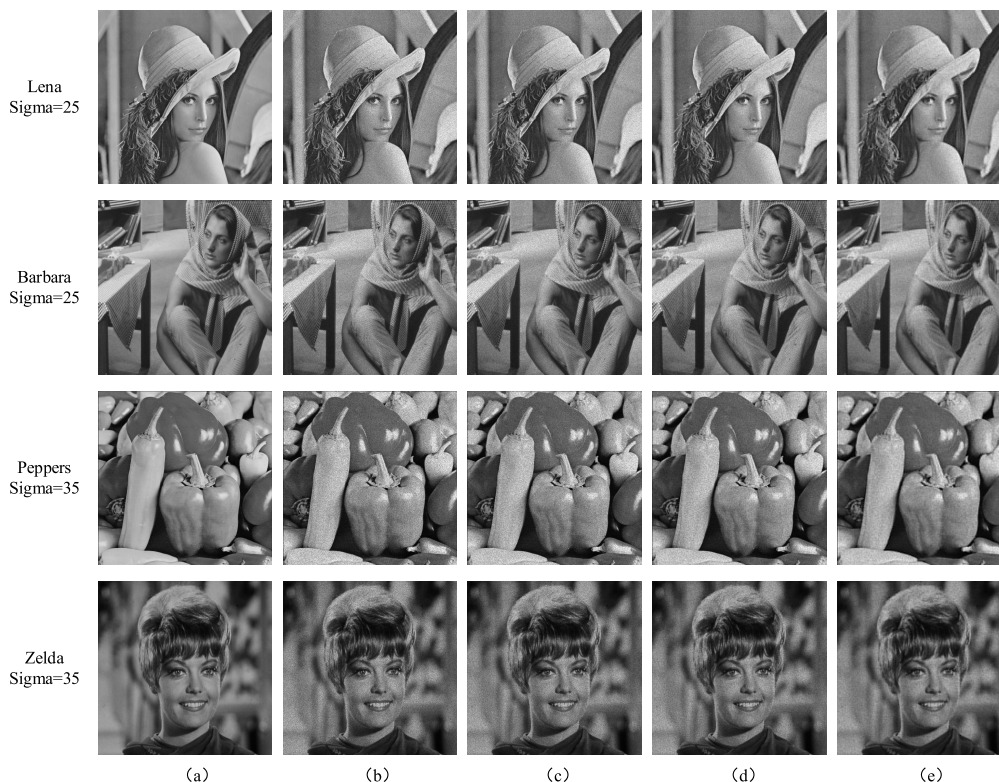
FIGURE 10. Results of image noise removal using 2D 8 \times 8 DCT+IDCT. (a) Original image. (b) Image with multiplicative noise added. (c) Light filtering mask. (d) Moderate filtering mask. (e) Heavy filtering mask.
