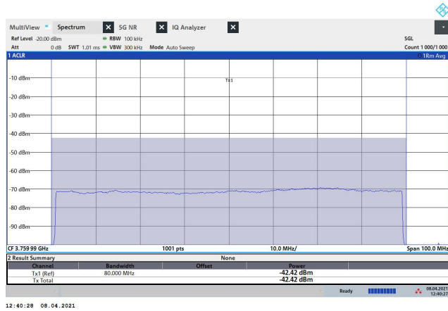
FIGURE 7. CP measurement in Rome in download full-loaded frame condition.
