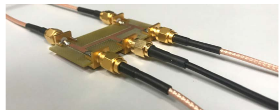
FIGURE 5. Four-way power divider used for phase synchronization of the SDR Array.
