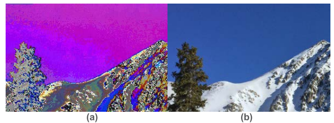
FIGURE 15. Received images in the presence of interference using interference cancellation weight from: (a) AOSMI and (b) GA. The transmitter was not synchronized to the receiver in either case.
