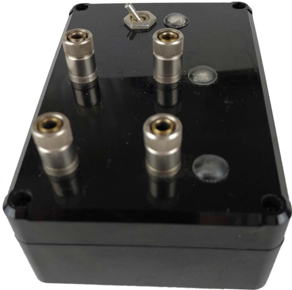
FIGURE 2. Aid used for measuring diodes. The aid has been created by a developer with blindness. Its internal connection is realised using a miniature screw terminal block.
