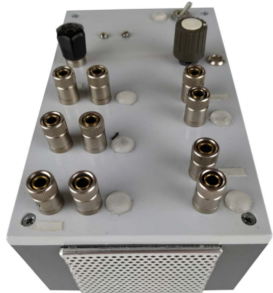
FIGURE 3. Sound measuring equipment for resistance estimation, diode testing, voltage identification and signal monitoring.
