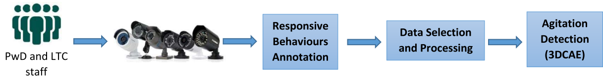
FIGURE 3. Pipeline for detecting agitation from videos.
