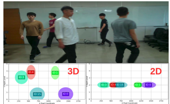
FIGURE 6. Bird's-eye view in 2D and 3D tracking state spaces. Each contour in the diagram represents a tracked object. In 3D space, each track can be effectively differentiated given their positions. However, in 2D space, objects are squeezed together, and it is difficult to differentiate them when they have ambiguous positions.
