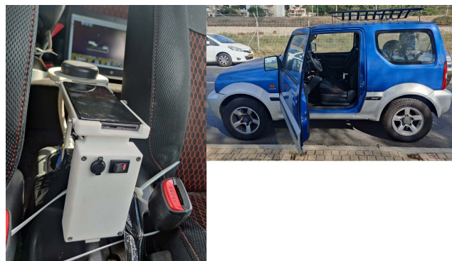
FIGURE 4. MRU and smartphone location inside the car.
