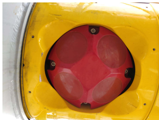
FIGURE 1. Teledyne DVL mounted on the Snapir AUV.
