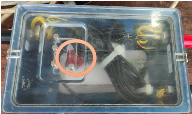
FIGURE 2. VN-100 inside the case, the sensor is marked by a red circle.
