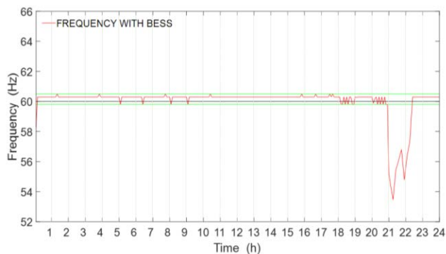
FIGURE 17. Frequency regulated by a BESS.
