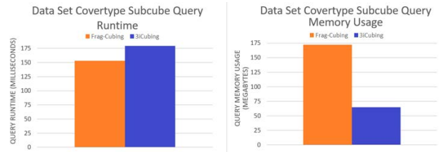
FIGURE 13. Forest Covertype data set average subcube query runtime and subcube query memory usage.
