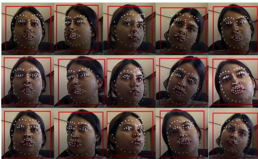
FIGURE 5. Real-time detection with top row at 300 epochs, middle row at 500 epochs and last row at 900 epochs.
