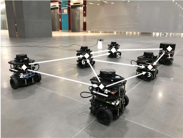
**FIGURE 3.** Robots in the experiment in the case of constant maneuvering: robots 1 and 2 are in Group A; their positions are estimated in a 2D plane in advance. Other robots are in Group B that measure the relative measurement, and the directional arrows represent information transmission links.
