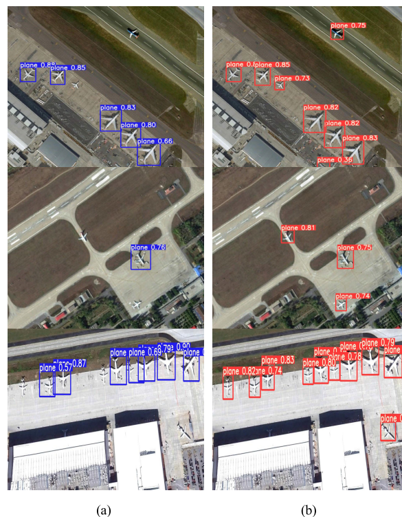
FIGURE 12. Comparison of detection results between YOLOv5 and improved YOLOv5. The detection results of YOLOv5 are shown on the left and the results of our method are shown on the right.
