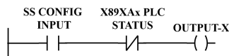
FIGURE 18. Inhibited to open (IHO) subset control logic implementation in PLC for isolator.
