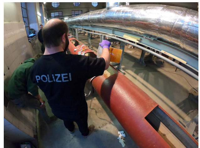
(b) Dumping of harsh industrial waste with different pH and conductivity characteristics to the wastewater stream by a German Law Enforcement Agent.
