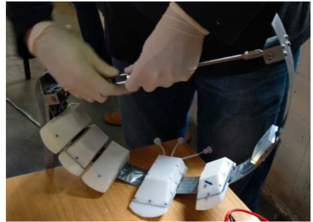
(a) IoT device assembly before testing. Modules from left to right: main module, two battery modules, sampling module and EC module.
