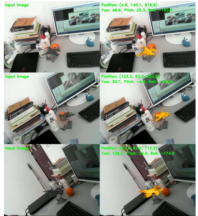
FIGURE 7. 3D tracking results for an aircraft model. Left: input image; Right: 6-dof tracking results. The 3D CAD model of the aircraft is rendered according to the estimated pose parameters and superimposed on the original image. The estimated 3D position and orientation are also displayed in the image.
