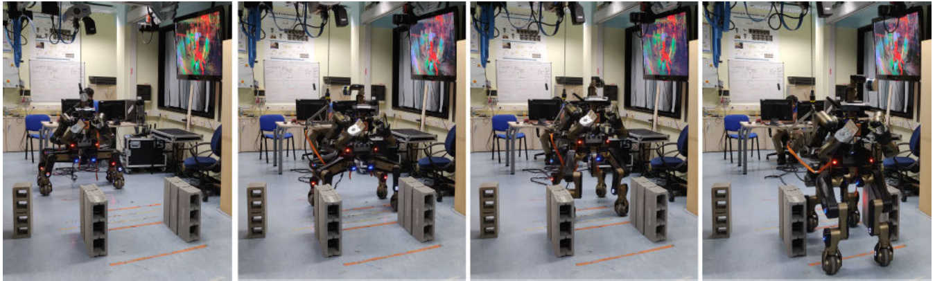
FIGURE 12. Sequence depicting the CENTAURO robot narrowing into the space in between the tall bricks to reach outside the narrow passage.
