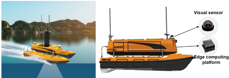
FIGURE 1. The ME120 USV with visual sensor and edge computing platform. The edge computing platform refers to NVIDIA Jetson AGX Xavier Developer Kit (or similar edge computing platform). Which supports NVIDIA Jetpack, DeepStream SDK, and other Deep-Learning software packs, including CUDA, cuDNN, TensorRT, etc.
