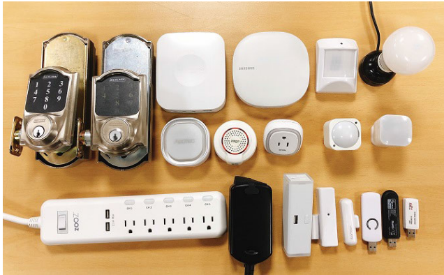
FIGURE 7. Z-Wave devices used for experiments. Clockwise from the top left: Schlage door lock BE468, Schlage door lock BE469ZP, Samsung SmartThings Hub, Samsung ConnectHome, Linear Motion Sensor, Linear smart LED bulb, Aeotec ZWA008 motion sensor, Aeotec ZW100-A motion sensor, Fibaro wall plug, Dome siren, Aeotec siren, SiLabs UZB-7 controller, Zooz S2 USB Stick, Aeon Labs Z-Stick Gen 5, Aeotec contact sensor, Linear contact sensor, Zooz S2 double plug with USB, Jasco Plug-in smart switch, and Zooz power strip.
