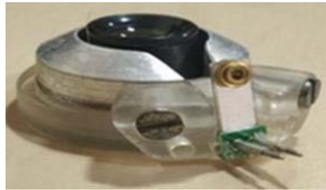
FIGURE 2. Embedment of vibration sensor on gonioleins.
