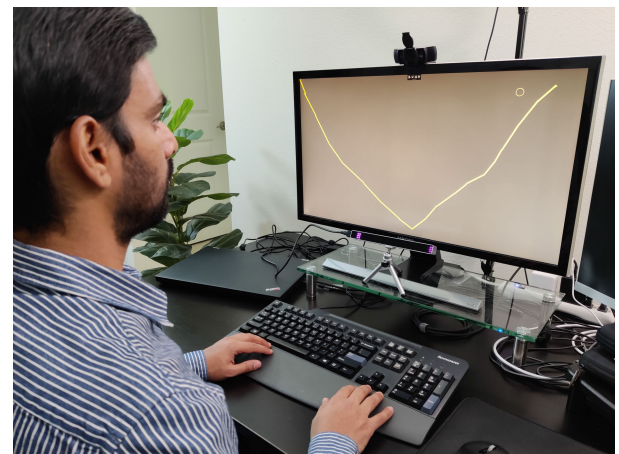
FIGURE 3. User study setup: a user is sitting in front of a computer with an eye tracker placed below the screen. The user has drawn the G4 gesture. The circle on the screen shows the current gaze location.
