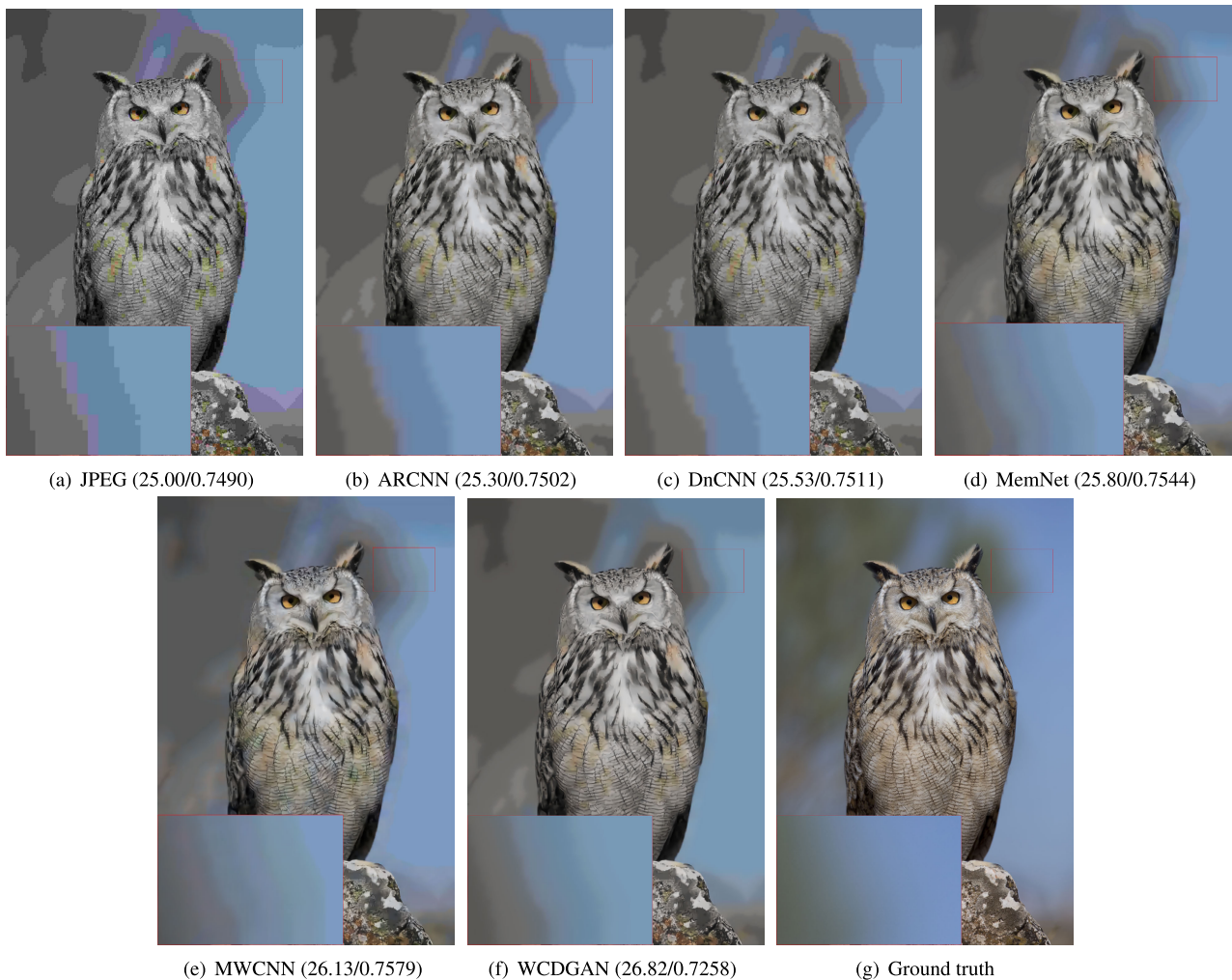
FIGURE 10. Visual comparison in 'Owl' (validation dataset of DIV2K) with quality factor 5 (PSNR(dB)/SSIM).
