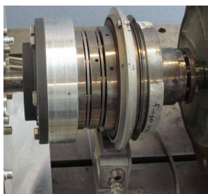
FIGURE 22. Torque and speed sensors mounted in between the two-in-one-motor system and the load machine.
