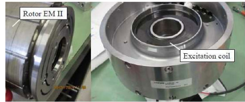
FIGURE 19. Electromagnetic clutch coupling EM1 and EM2.
