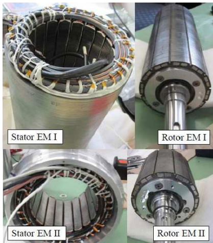
FIGURE 18. Photos of the stators and rotors of EM1 and EM2.
