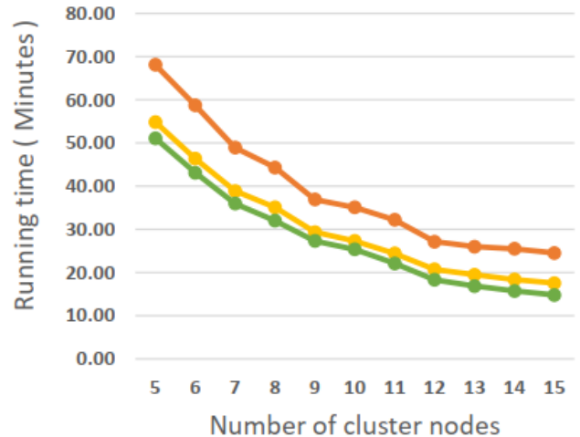
FIGURE 6. The running times of MPFP, BPFP and EBFPF algorithms in the webdocs dataset on different number of cluster nodes.
