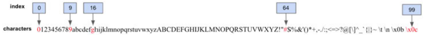
FIGURE 2. The characters dictionary with 100 ASCII characters which are widely used in URLs.
