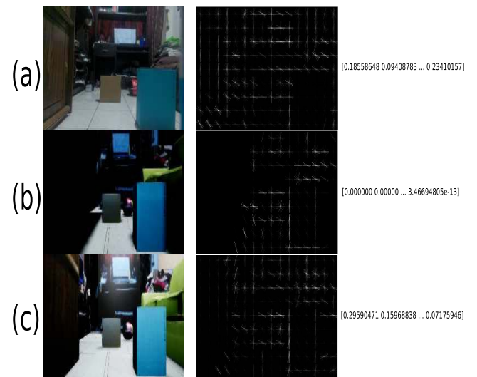
FIGURE 5. Histogram of oriented gradients for each sample. (a) Physical world. (b) Virtual representation with an essential light source. (c) Virtual samples with lights and materials.
