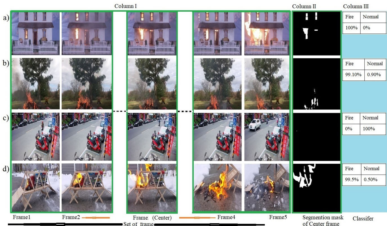
FIGURE 17. Set of sample frames in video clips. a) The fire was increasing in a successive frame, b) the fire was almost consistent, c) video clip contained red color banner, and d) first, the fire was growing later shrinking.
