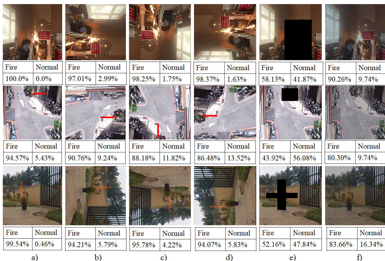
FIGURE 20. Robustness of the proposed fire detection under various conditions, top row: NTUST, middle row: small-sized fire, and bottom row: Foggia dataset. a) No rotation, b) Clockwise 90, c) Clockwise 180 d) Clockwise 270, e) occlusion, and f) adding noise to video.
