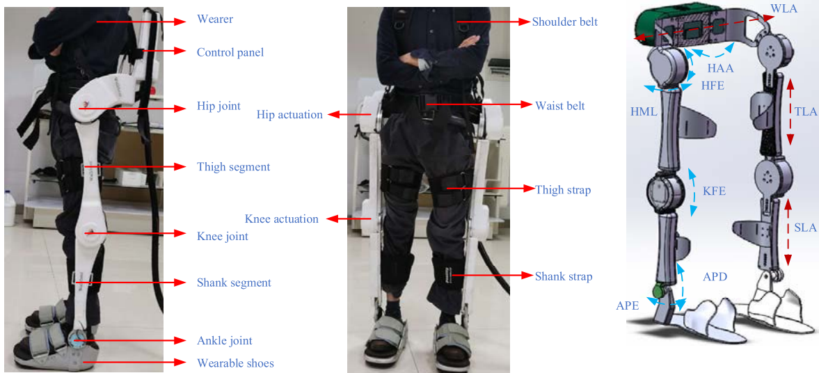
FIGURE 1. The structure of the exoskeleton. HAA = hip adduction/abduction, HFE = hip flexion/extension, HML = hip medial/lateral rotation, KFE = knee flexion/extension, APD = ankle plantarflexion/dorsiflexion, APE = ankle pronation/external rotation; WLA = waist length adjustment, TLA = thigh length adjustment, SLA = shank length adjustment. The HFE and KFE DoFs are powered by DC motors and other DoFs are passive. The waist part can be adjusted up to 38cm. The length of the thigh and shank segments can be adjusted to fit the human user in the height of 155cm-185cm.
