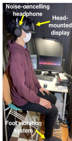
FIGURE 1. Overview of the virtual walking system. Visual stimuli were presented on an HMD controlled by a computer, which also controlled and presented tactile stimuli through the vibration system on the feet. A noise cancelling headphone was used to eliminate sound from the vibration system.
