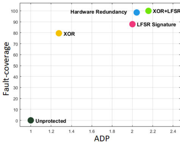
FIGURE 9. Fault-coverage versus area delay product (ADP) for each countermeasure scheme.
