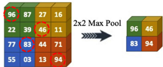
FIGURE 3. An example of a 2 \times 2 max pool operation is shown. A 4 \times 4 matrix is divided into four 2 \times 2 matrices and down sampled to half the size by neglecting all the low-magnitude elements and retaining the highest magnitude element among the 2 \times 2 group.
