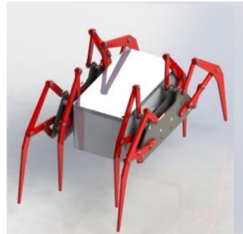
FIGURE 1. CAD design of paired four-legged amphibious robot leg position.
