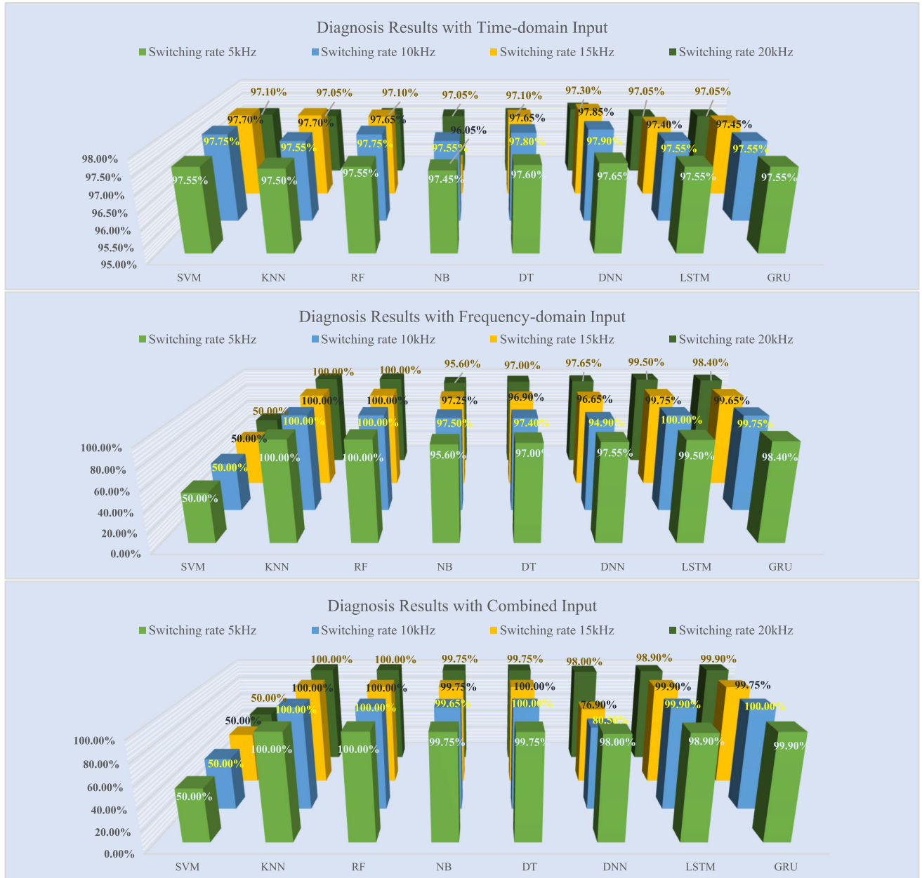
FIGURE 12. Arc diagnosis results for the single-phase inverter with SPWM at 5 A under different input types.
