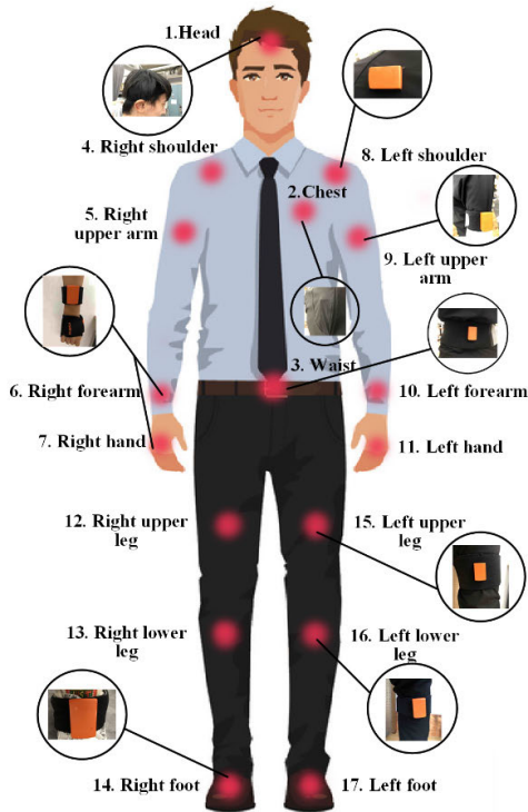
FIGURE 3. Locations for sensors worn on human body (with image of selected sensors). For generality, the Xsens sensors are attached to the commonly worn placement of the human body, such as the wrist, middle of thigh (as the pocket position), middle of forearm and so on.
