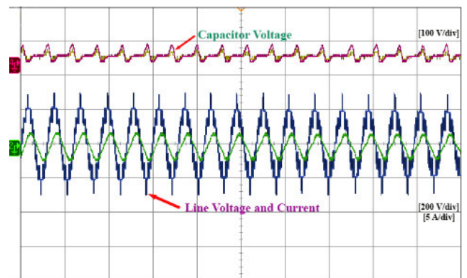
FIGURE 20. Experimental results of SM capacitor voltage and line components.
