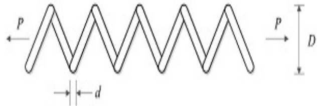
FIGURE 12. Schematic view of the tension/compression spring problem.
