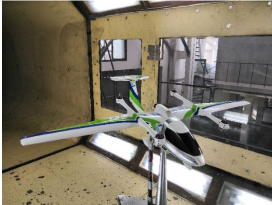
FIGURE 5. A 16.67% scale tunnel model of ET120 in a low-speed wind tunnel.
