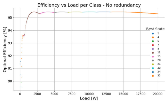
FIGURE 14. No redundancy case, most efficient state per load.
