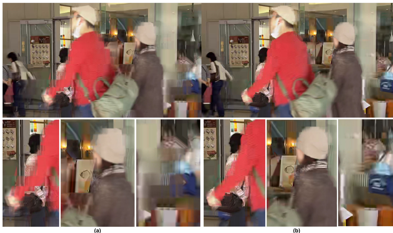
FIGURE 8. Visual quality comparisons of (a) the existing R- \lambda model at 456.74 Kbps and (b) the proposed algorithm at 452.59 Kbps on frame #85 of the "BQMall" sequence.
