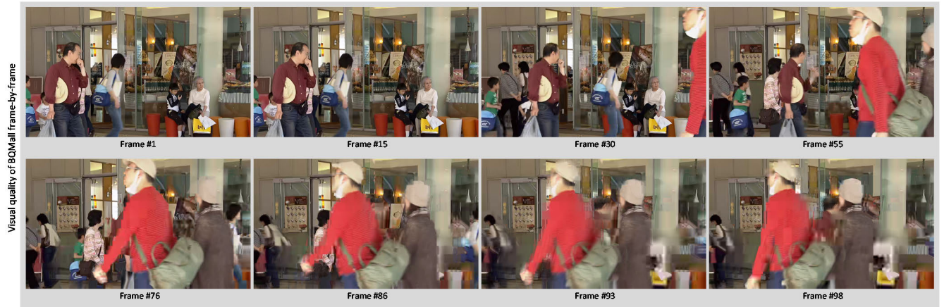
FIGURE 2. Subjective quality of the “BQMall” test sequence with the rate control in HEVC enabled.
