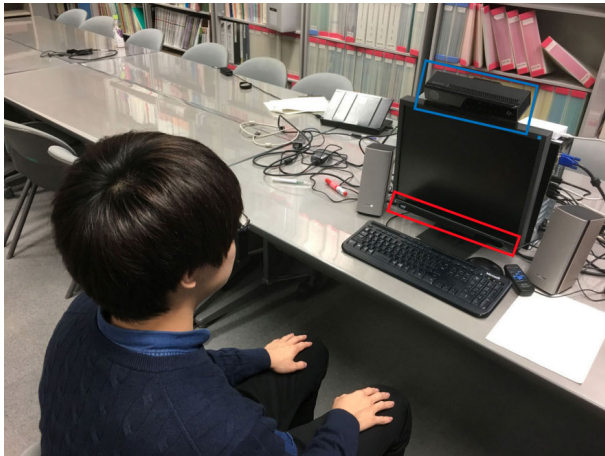
FIGURE 1. Experiment's environment. Red and blue squares indicate a sensor of Tobii Eye Tracker 4C and that for OpenPose, respectively.
