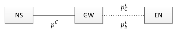
FIGURE 6. End-to-end link comprising a LoRa radio connection which is indicated as a dashed line and a cable-based connection which is indicated as a solid line. The notations EN, GW, and NS represent end node, gateway, and net server, respectively.
