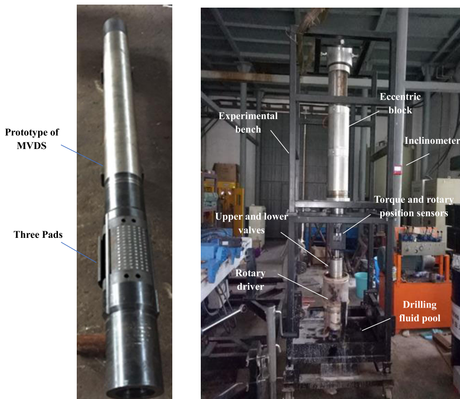
FIGURE 18. Prototype of MVDS and Eccentric block response test bench.
