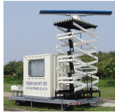
FIGURE 5. Bird surveillance avian radar systems developed by CAAC.
