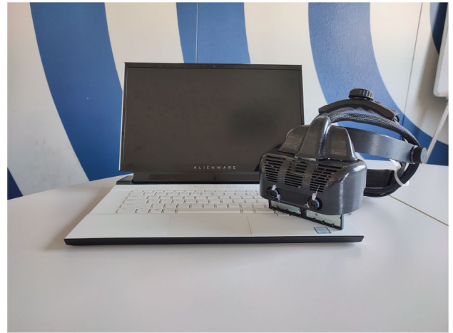
FIGURE 1. The laptop on which the computing unity runs and the custom-made hybrid optical/video see-through head-mounted display.
