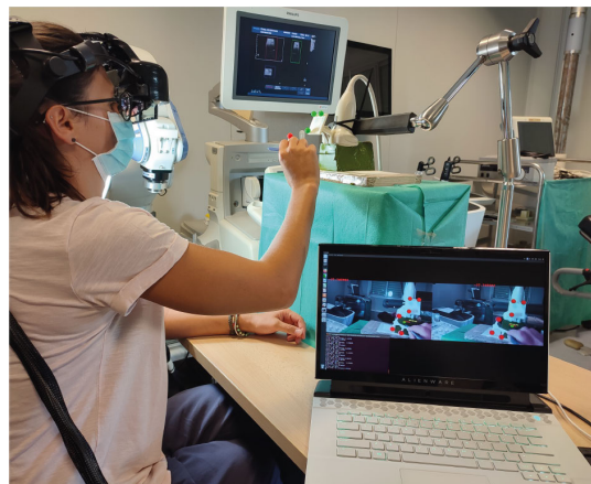
FIGURE 10. Experimental setup designed for the surgical access with a user performing the task. On the lower right corner, the augmented images projected onto the displays, whereas on the ultrasound system monitor the real-time ultrasound acquisition.
