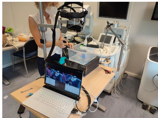
(a) The experimental setup. Note the three flexible mounting arms on which respectively the visor, the US probe, and the scalpel are mounted; the tray containing the comb; the computer with the application running.
