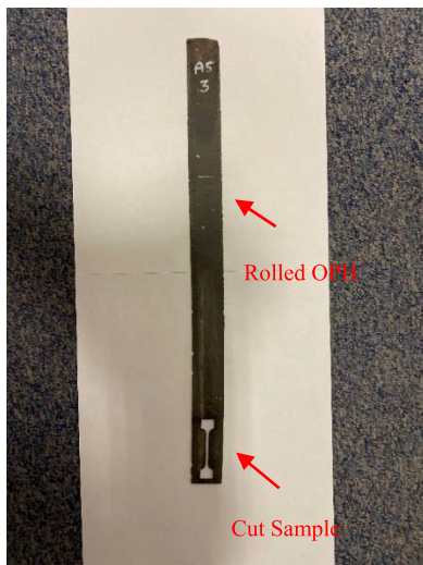
FIGURE 3. Position of cut samples direction of rolling.
