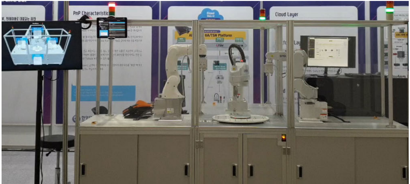
FIGURE 10. Demonstration of the plug-and-produce manufacturing system. (Two robots were running, as shown by the green indicator lights.)
